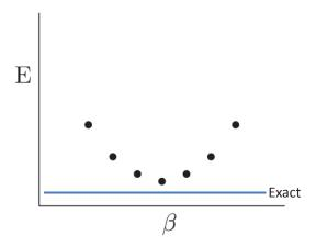
Since  $\beta$  appears in  $\Psi$  as a nonlinear parameter, the entire calculation must be repeated for each value of  $\beta$ . However, the minimum becomes progressively lower as the basis set is enlarged.
